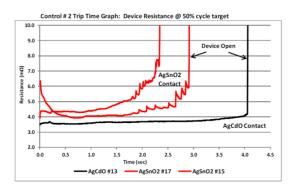
These include higher contact erosion, contact resistance and bulk resistance as well as greater temperature rise. Overall, AgCdO contacts last longer and have properties that make them ideal for safety-related applications where device failure must be minimized. Products made with substitute contacts may be more susceptible to failure in the dangerous welded-closed state more often than are AgCdO contacts.
