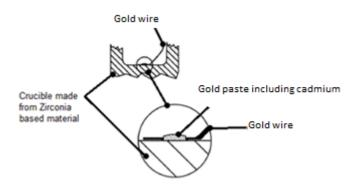
The passage of  $O_2$  ions becomes possible at high operating temperatures as at the operating temperature of the transducer - the zircona - becomes conducting. This therefore produces a voltage across the electrodes, the magnitude of which is a logarithmic function of the ratio of the  $O_2$  partial pressures of the sample and reference gas.
